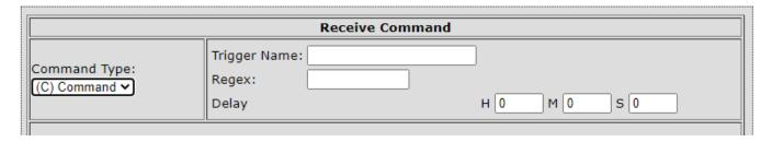
The Command Trigger Receive section is very simple from a UI standpoint but more complicated from a user standpoint. As always, you first start by giving the Trigger a name that describes its function.
