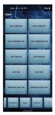
Notice that the buttons that were added to the Control Panel are identical to what shows up on the app. This is how you design the user interface on the mobile app.
