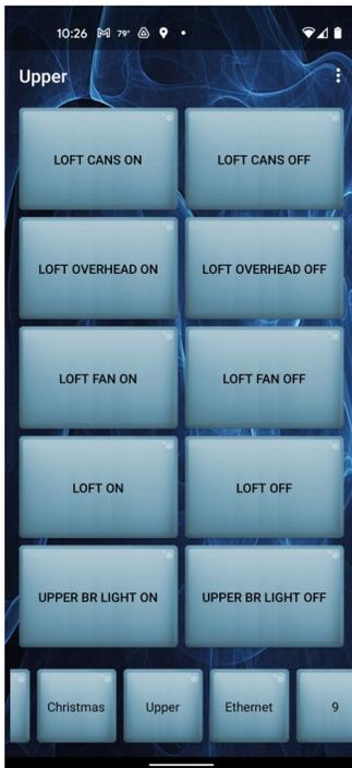
Notice that the buttons that were added to the Control Panel are identical to what shows up on the app. This is how you design the user interface on the mobile app.
